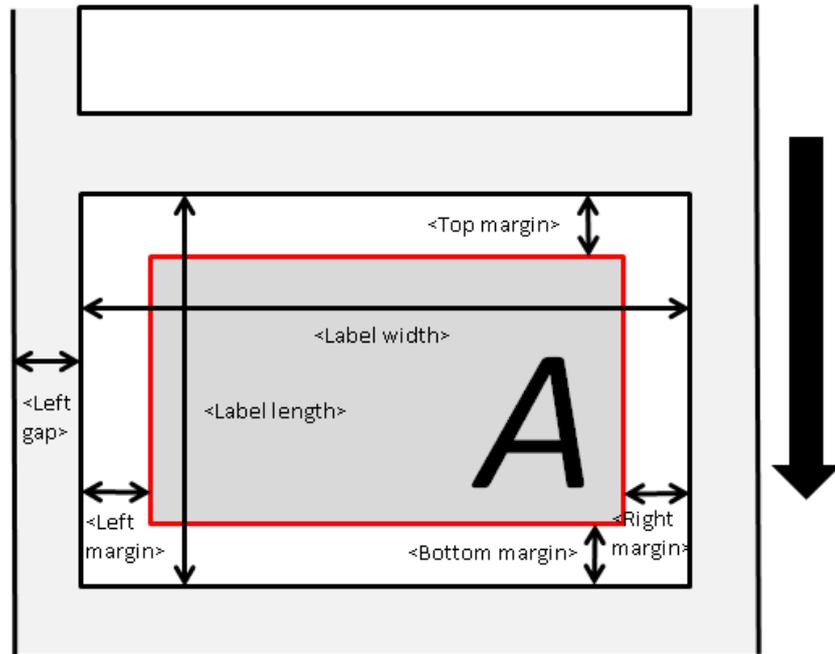
Figure 3-2 Die-cut Label (Gap) Layout
