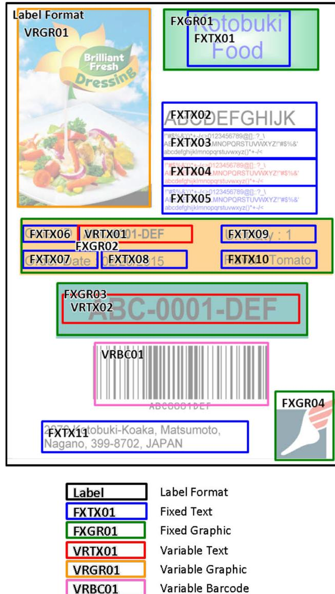
Figure 5-2 Divided Result of the Sample Label into Fixed-Fields and Variable-Fields
