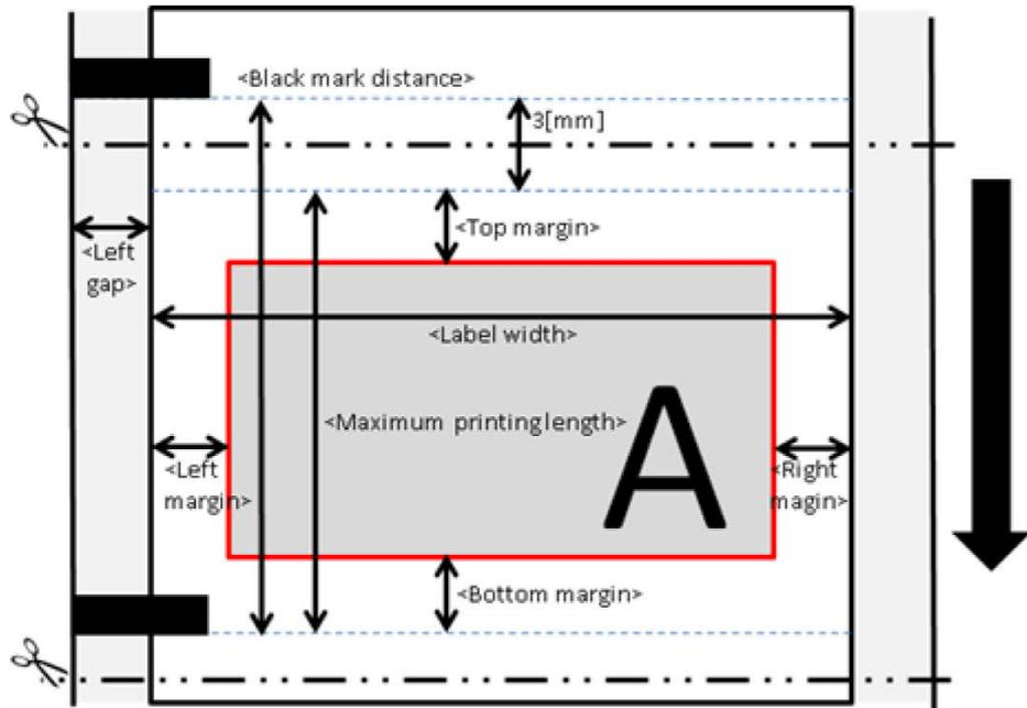
Figure 3-5 Continuous Label (BM) Layout
