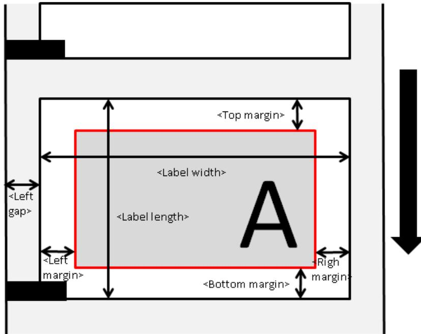
Figure 3-3 Die-cut Label (BM) Layout
